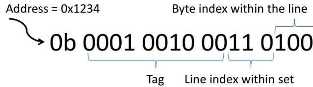
**Figure 5.1:** Breakdown of a 16 bit address for a cache of line length 8 bytes and a set size of 8 lines.
