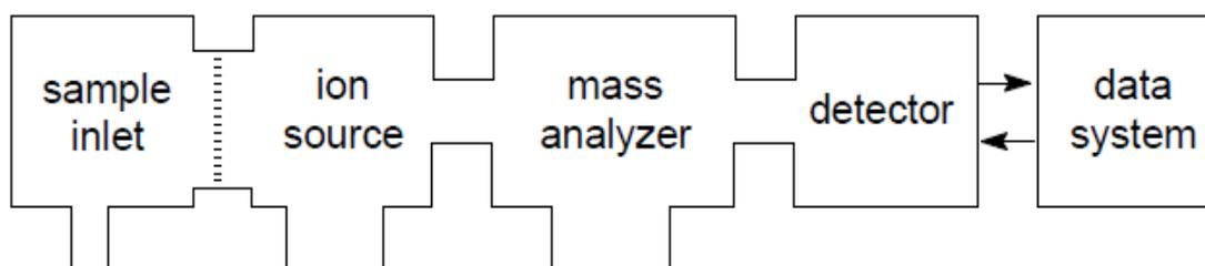
**Figure 1.6 Basic concept of mass spectrometry, reproduced from Gross<sup>96</sup>.**
