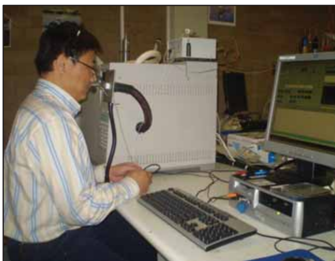
Figure 3.17 Operator at the odour detection port (ODP) using headset microphone and a control pad for intensity ranking.
