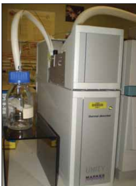
Figure 3.14 Direct headspace sampler showing sample vessel and thermal desorption unit (Markes International, UK).
