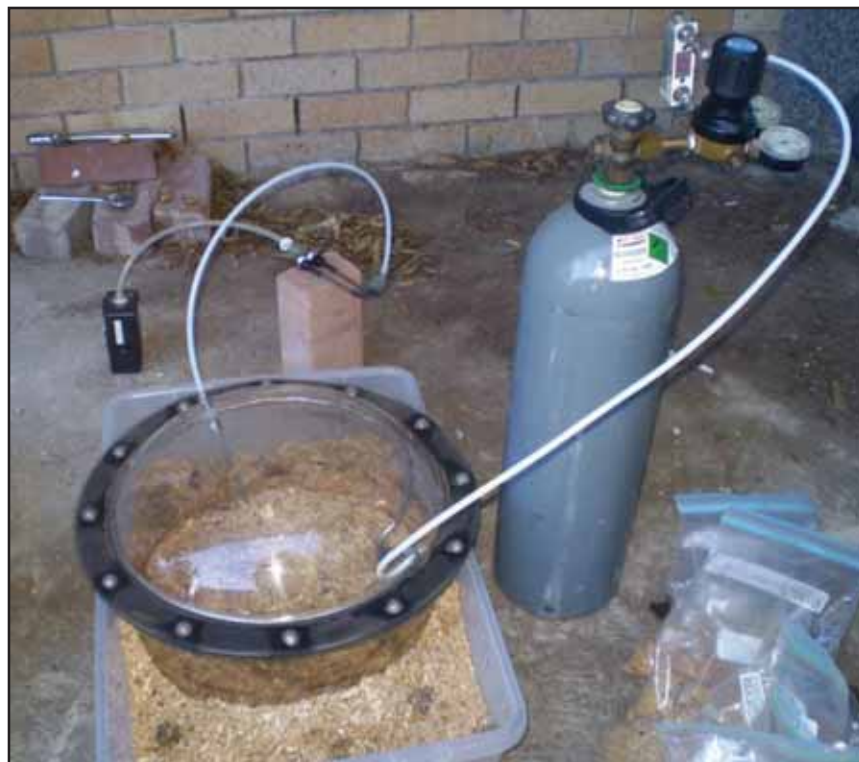
Figure 3.11 Sorbent tube sampling of litter material using a flux hood technique.
