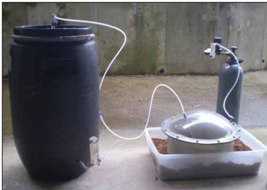
Figure 3.7 Olfactometry sampling using a flux hood and nitrogen purge.
