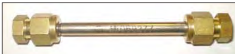
Figure 3.10 Example of sorbent tube, Tenax TA.
