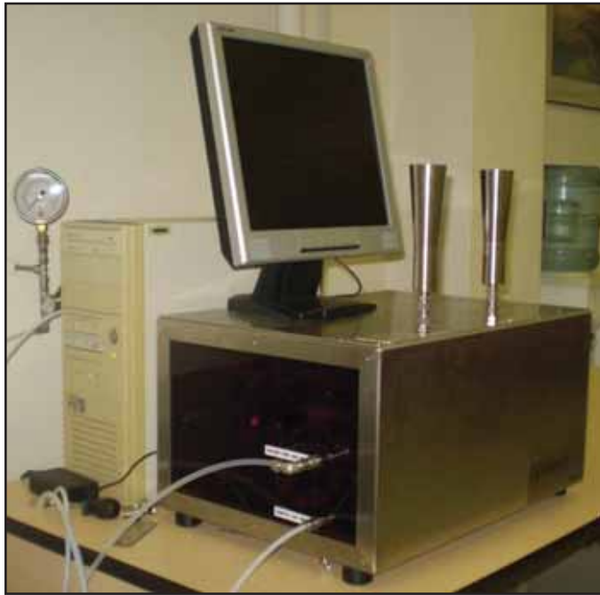
Figure 3.8 Forced choice dynamic dilution olfactometer set in the UNSW Atmospheric Emissions and Odour Laboratory.
