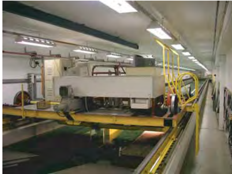
Figure 4.4: The Towing Tank and Carriage at The Australian Maritime College, Launceston, Tasmania ( Photograph by S. Robards )
