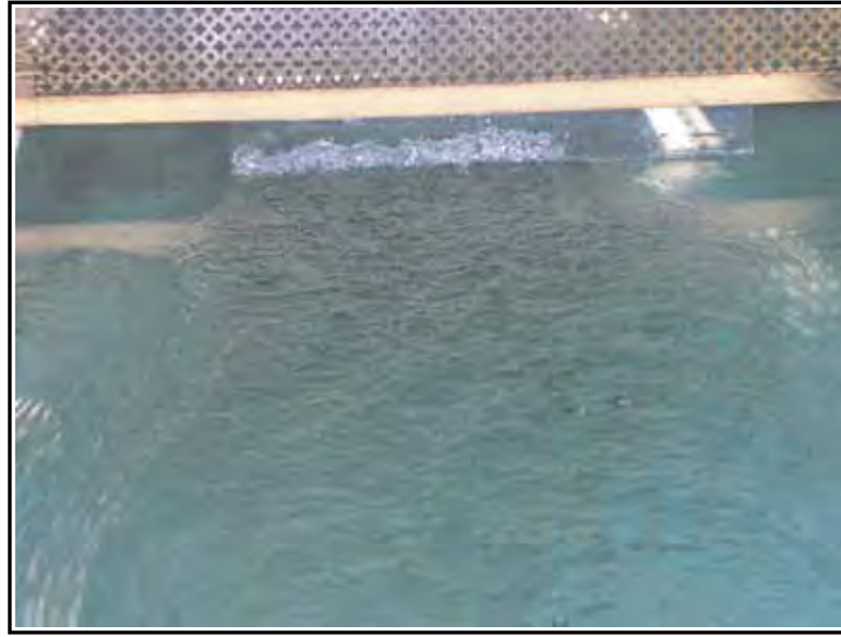
Figure 5.5: A Plastic Sheet Placed Just Touching the Water Surface was used to Roughen up the Previously Undisturbed Free Surface Without Creating a Major Depression in the Water.
