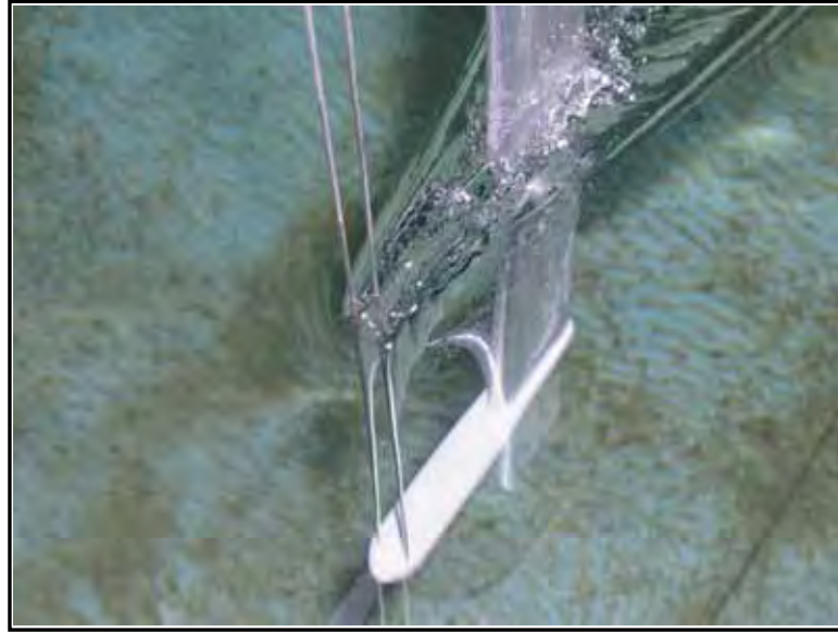
Figure 5.3: Flow Separation from Probe Wires at F_{PR}=22.04 (2.673 m/s)
