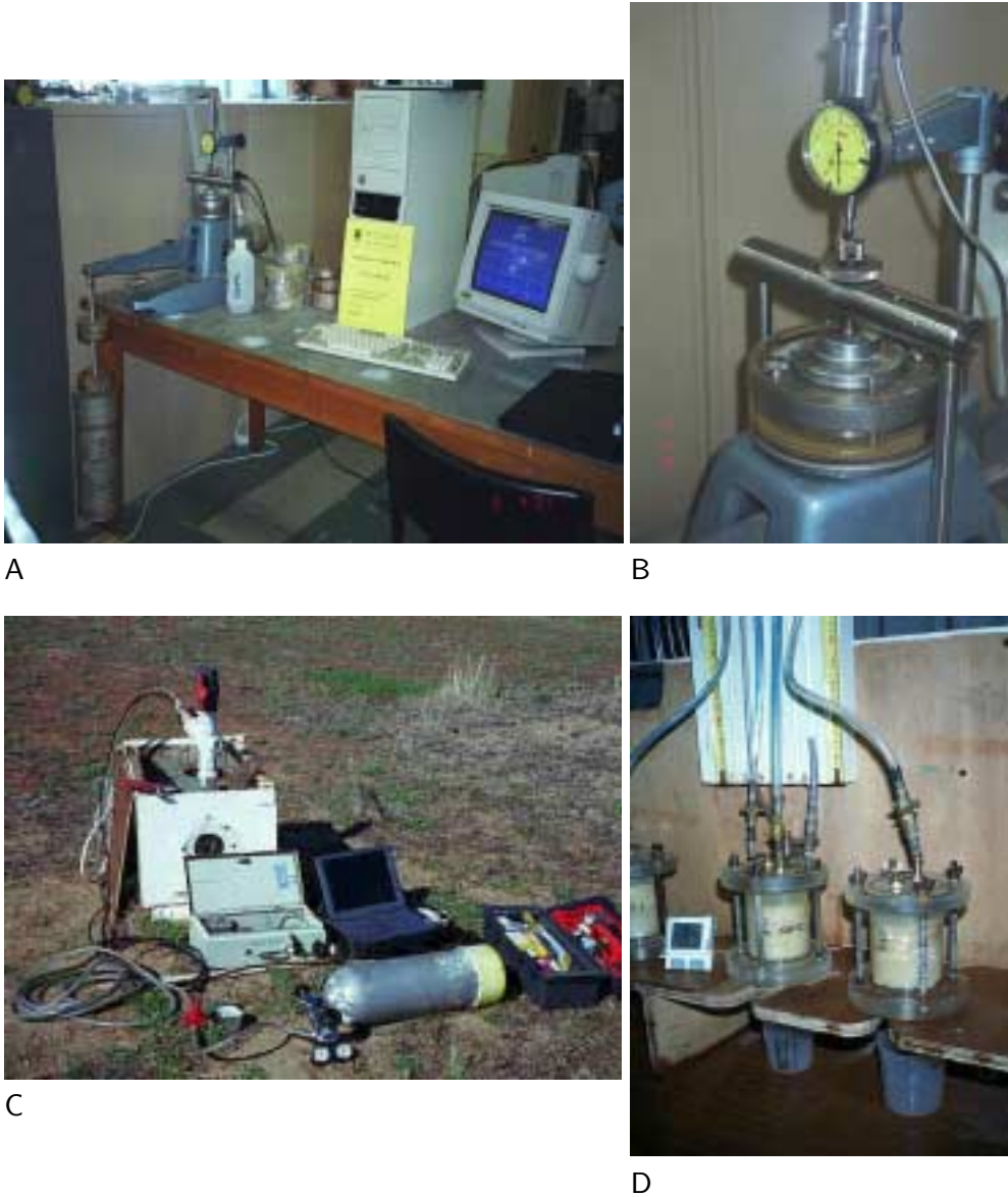
Figure 4.3: Permeability testing methods A Oedometer testing of consolidation. B Oedometer testing of core sample 2 cm thick by 7 cm diameter. C Slug testing of piezometers using compressed air. D Permeability testing of core samples by falling head permeater.
