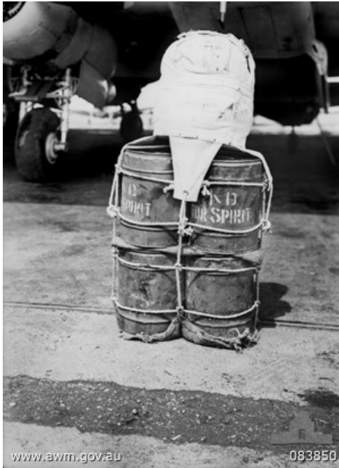
14. POL prepared for dropping. Cornsacks are used between and under the drums
