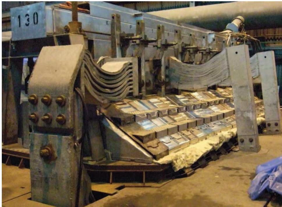
Figure 2.7: Modified Reynolds P19 cell design installed in Hamburg
