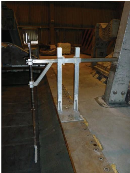
**Figure 5.1:** Ledge measurement system in a new cell
