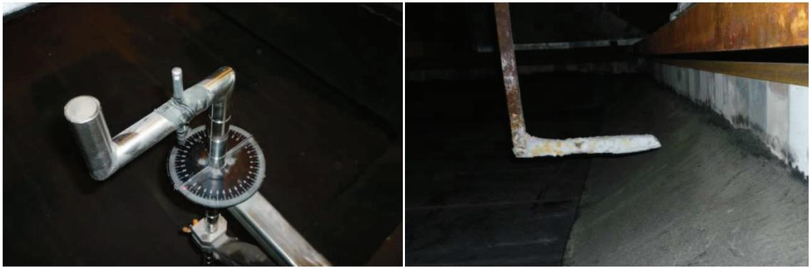
**Figure 5.2:** Dial used for determination of the angle (left) and hook inside the cell (right)
