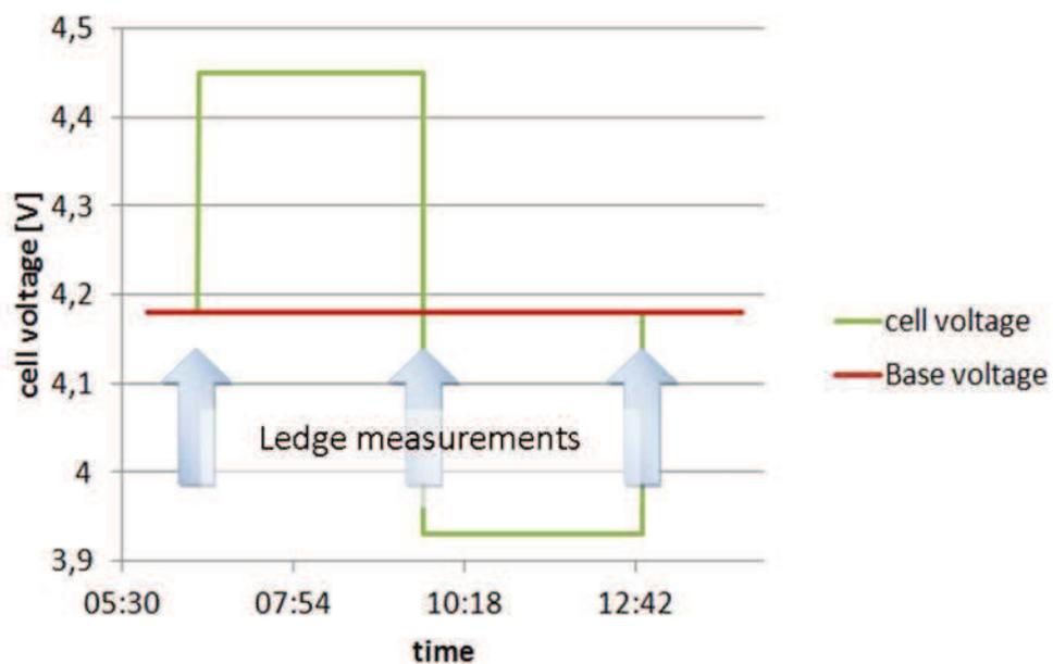
**Figure 5.24: Cell voltage over the experiment**
