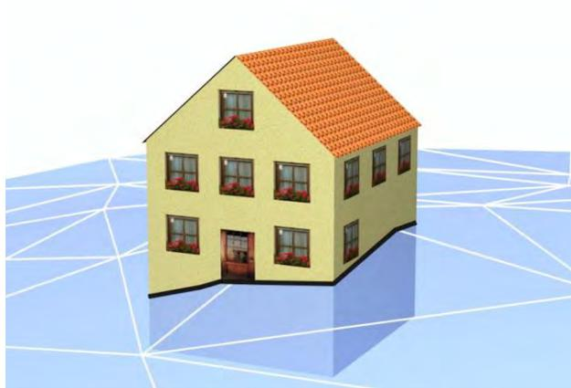
FIGURE 3.6: *TerrainIntersectionCurves* (TIC) in CityGML. The TIC is shown in bold black curve.
