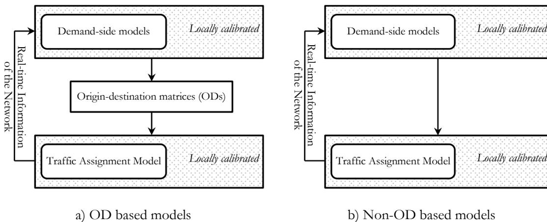
Figure 2-2 The linkage of ABM and TA in simulation
