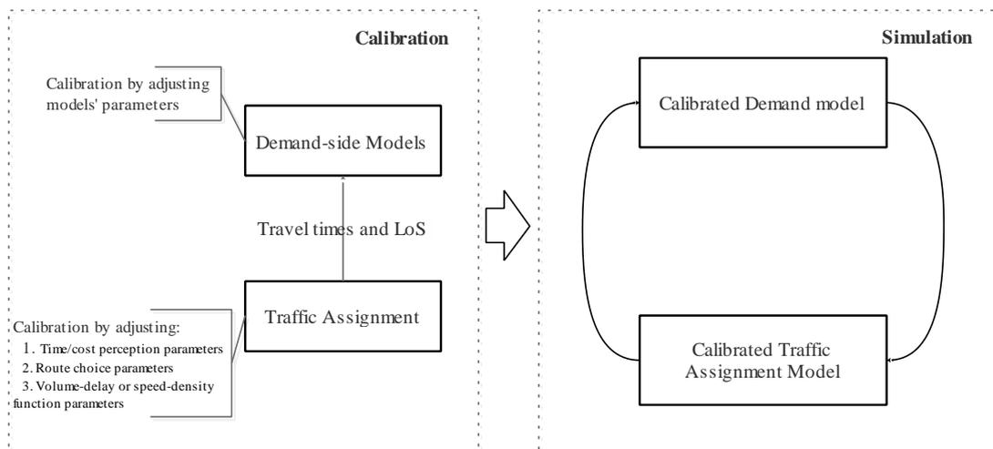
Figure 4-1 Conventional TPMS estimation, calibration and simulation processes
