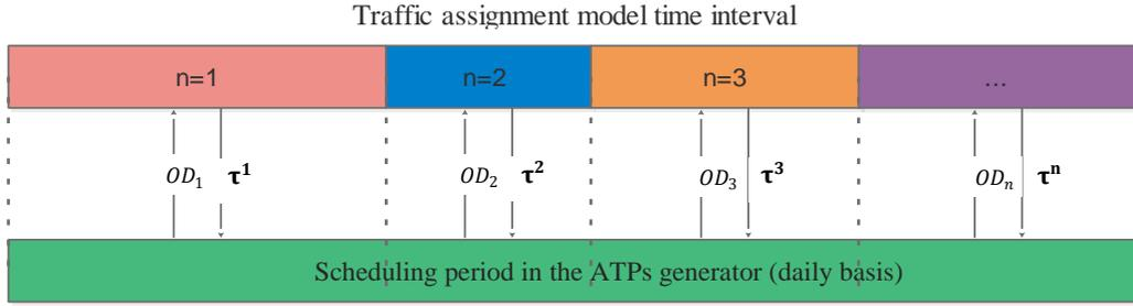
Figure 6-5 The interaction between the ATPs generator and traffic assignment model
