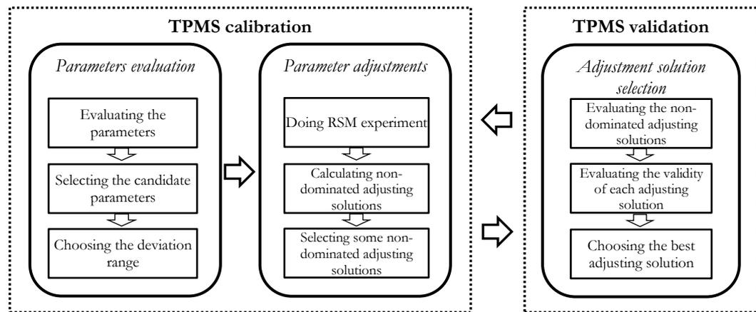
Figure 4-3 Proposed model structure for the calibration process
