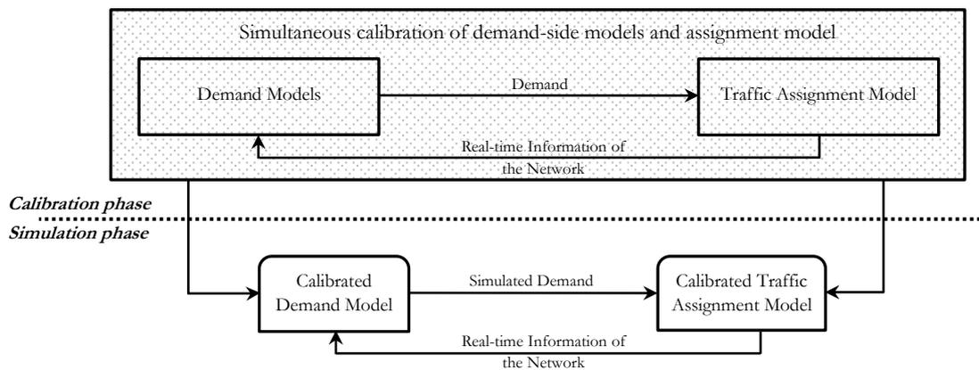
Figure 3-3 The desirable structure in developing a fully integrated transport model
