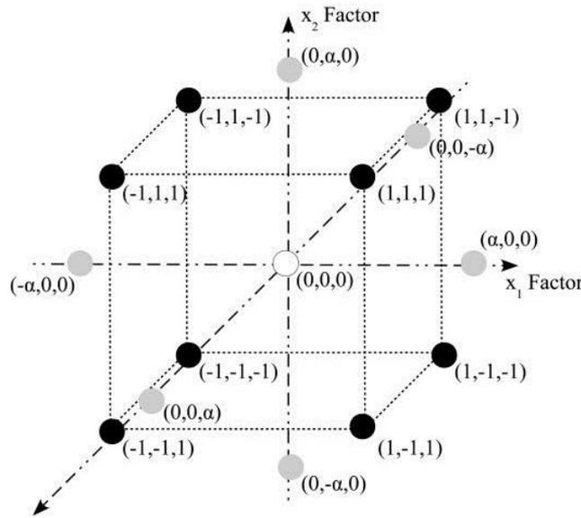
Figure 4-2 Schematic diagram of a three factor central composite design (CCD)
