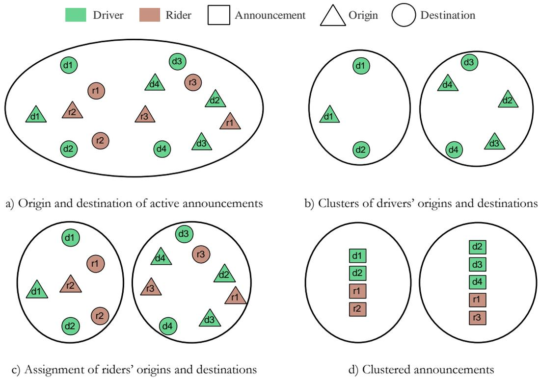
Figure 7-4 Illustration of the intersecting clustering algorithm with  $|N| = 2$
