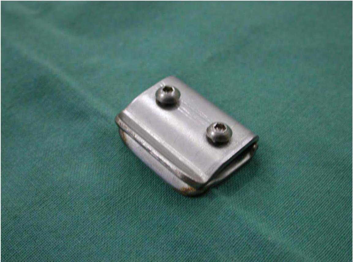
**Figure 13** The clamp mechanism used to fix the elastic wrap around the aorta.
