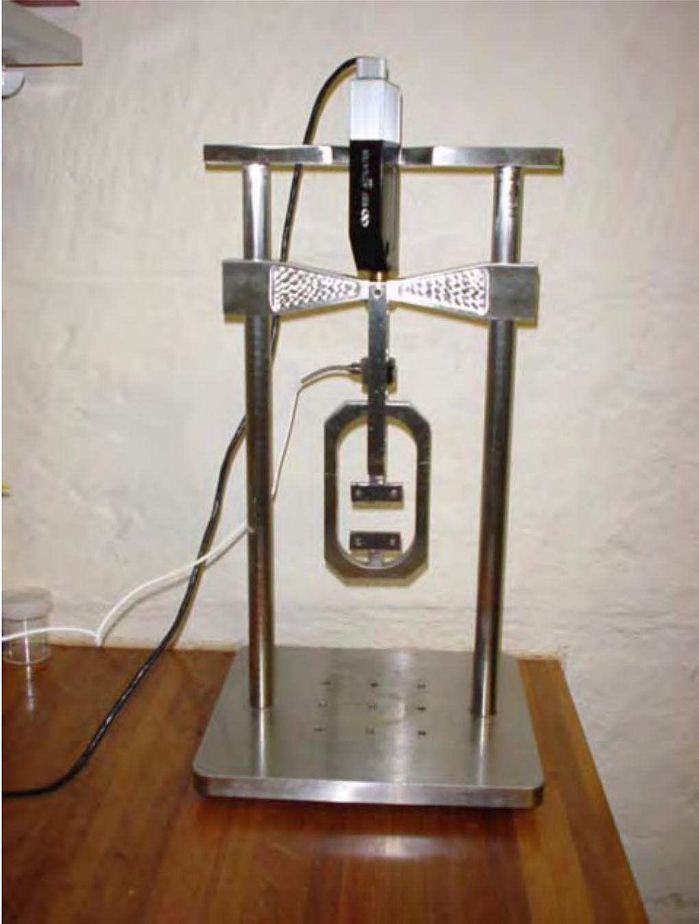
**Figure 124** Mach-1 micromechanical testing machine (Biosyntech Canada Inc., Quebec, Canada).
