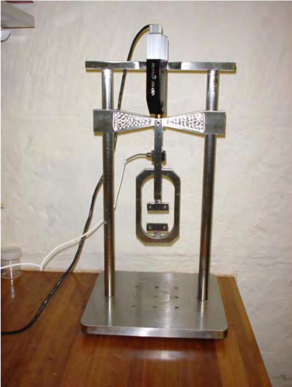
**Figure 91** Mach-1 micromechanical testing machine.
