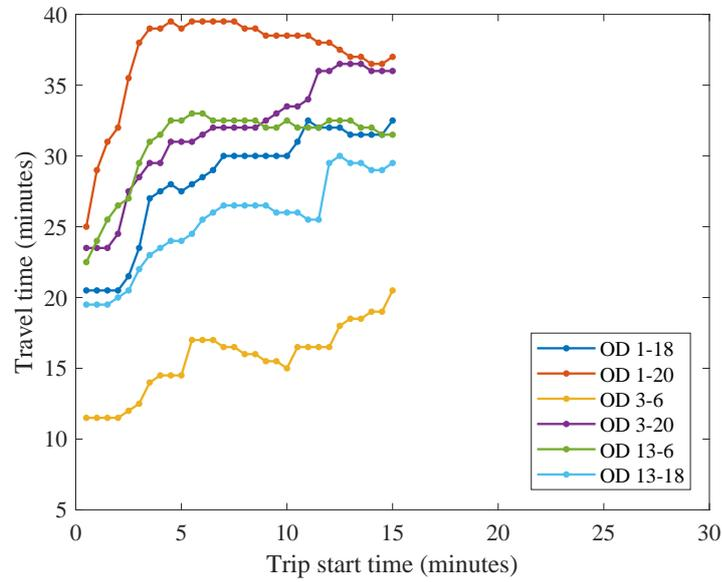
Figure 3.9: Travel times based on departure time (with wait time at origin)
