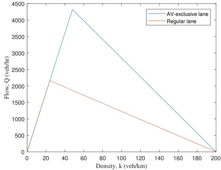
Figure 5.1: Fundamental diagrams of traffic flow for two lane types
