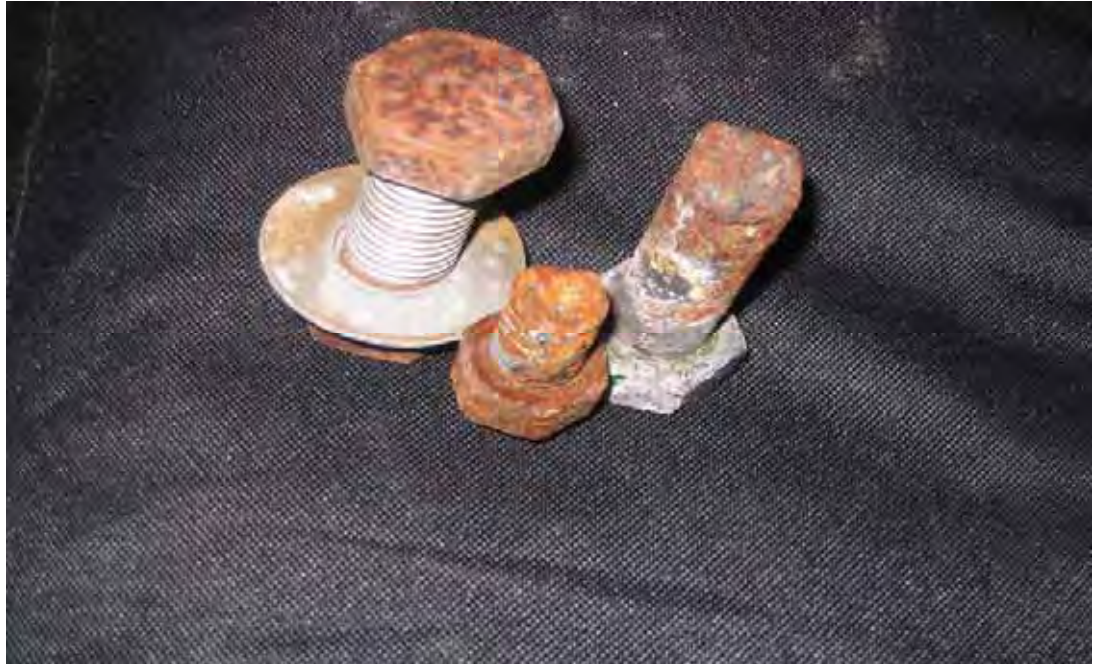
Figure 4.15 Bolts failed due to corrosion and cyclic loading.
