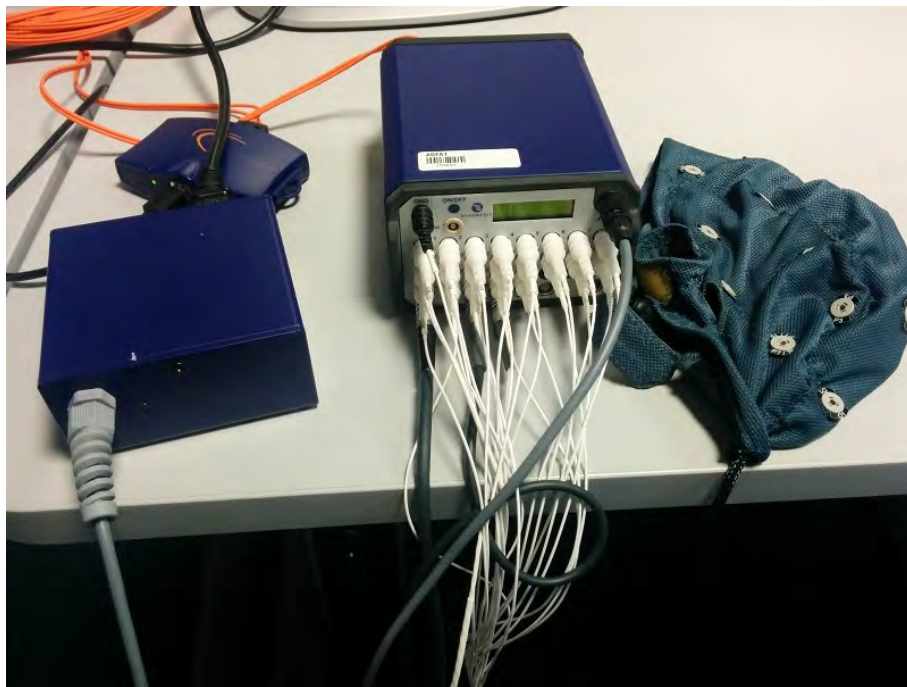
Figure 6.3: EEG Collection System and EEG Cap
