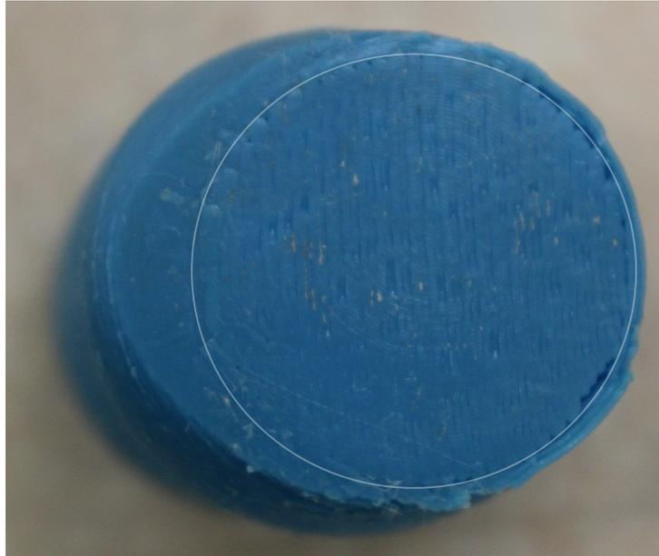
Fig. 5.21 Top view of cylinder compressed at large strains. Contacting surface has increased non-uniformly on the left side from initial surface highlighted in white.
