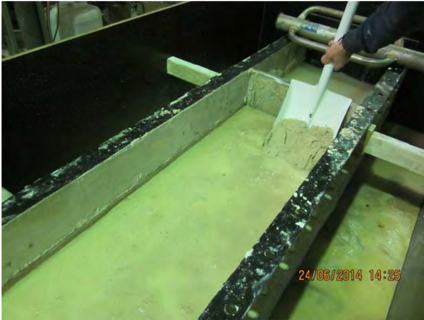
Figure 48-2 soil placed slowly from shovel through very shallow water
