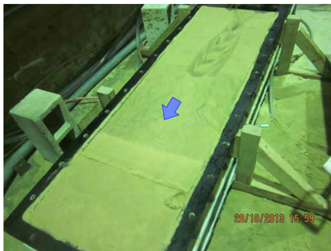
(c) Forward deepening had reached halfway before Test 25 was stopped; shown once lid removed
