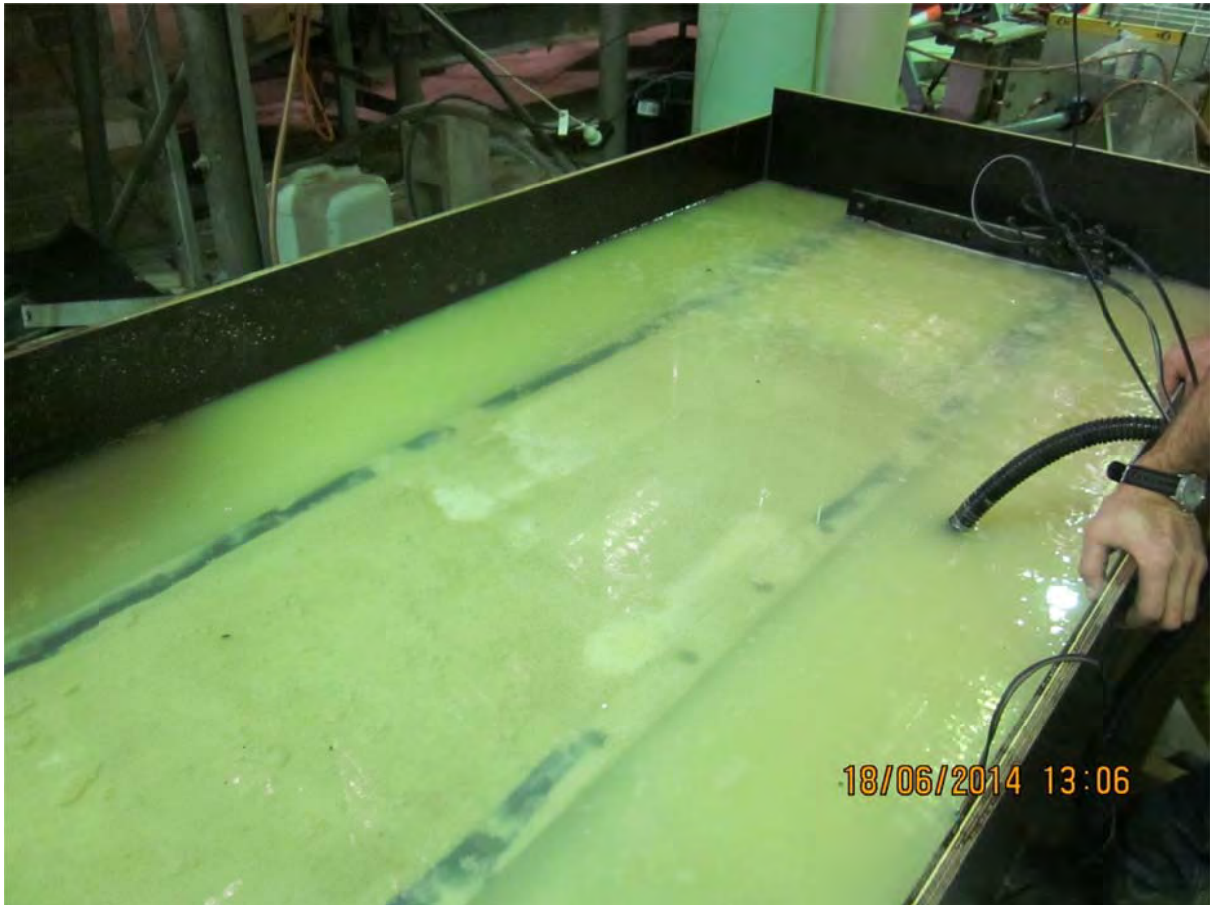
Pic 7: fine-grained concentrations at points of max vibration (under vibrator)
