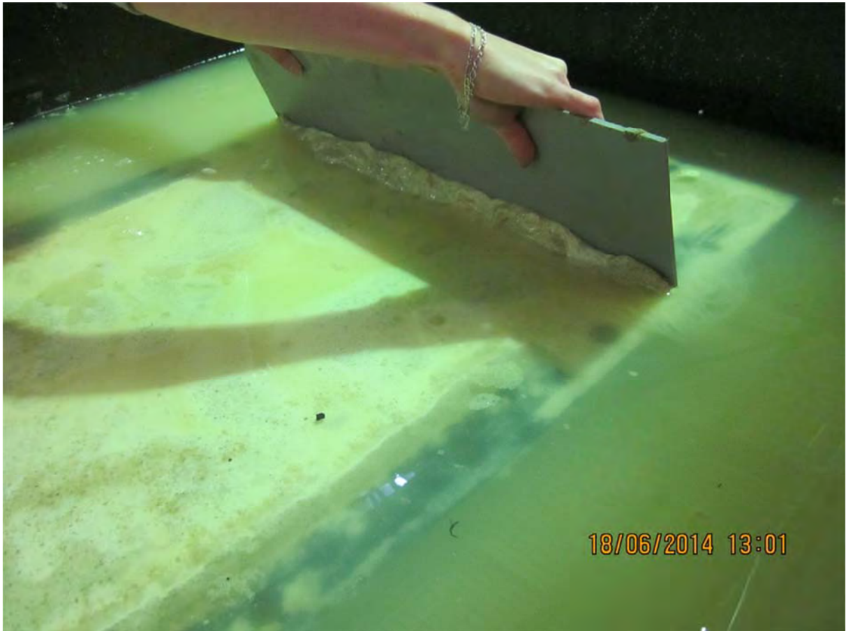
Pic 2: Screen off top surface of soil
