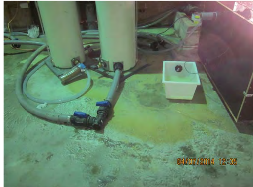
Figure 48-13 Soil carried out onto lab floor from flow leaving flume after failure
