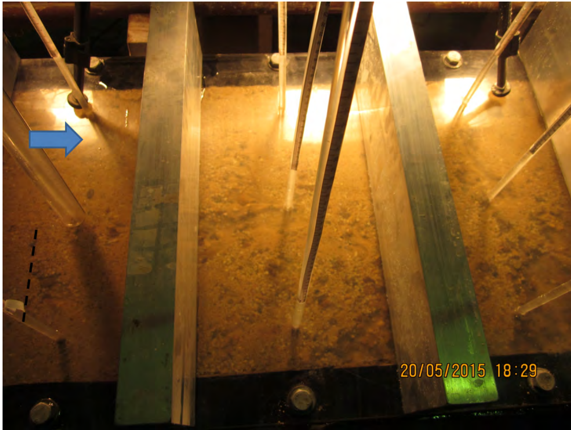
Figure 8.8: Channel and tip difficult to identify. Tip identified at dashed line. (blue arrow indicates direction of flow)
