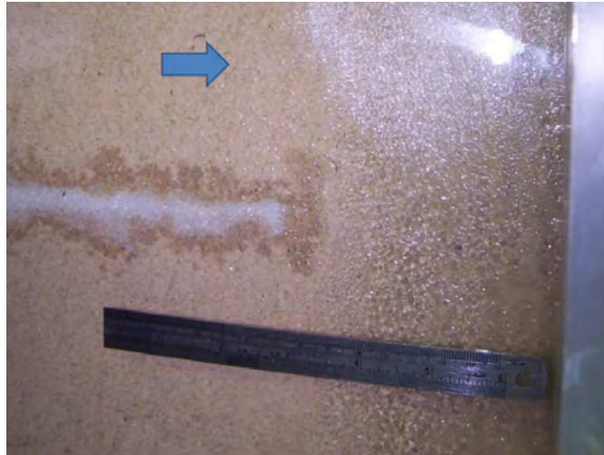
Figure 3.43: Sugar designed to dissolve upon saturation and leave open starter channel behind but starter channel collapsed upon dissolving (blue arrow indicates direction of flow)
