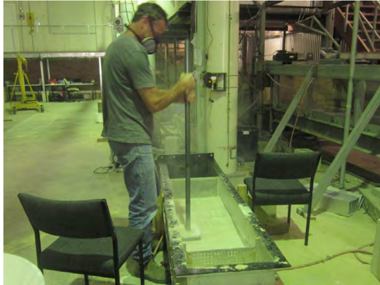
Figure 3.40: Air-born Sibelco 300g during tamping (and respirator use)
