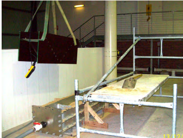
Figure 3.39: Sand rainer suspended by crane above flume
