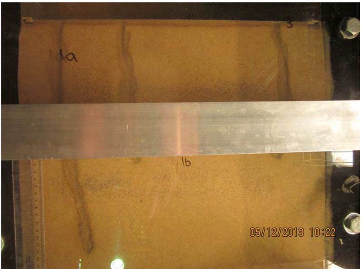
This photo shows the sand discolouration at the u/s end.
