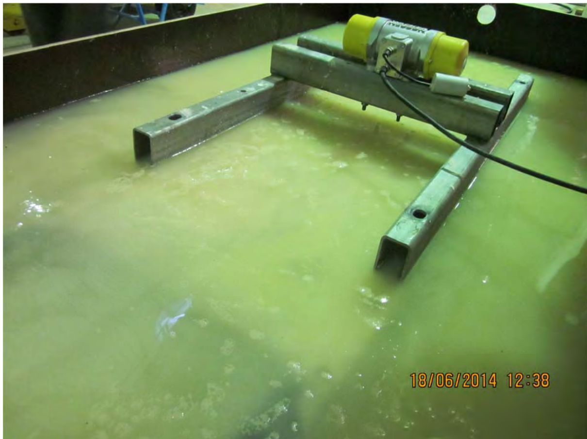
Pic 1: last vibration with flume full of soil and water just over top of flume
