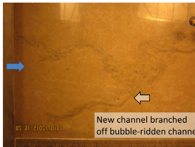
Figure 8.12: Air bubbles in channel and new channel which branched off existing (blue arrow indicates direction of flow)
