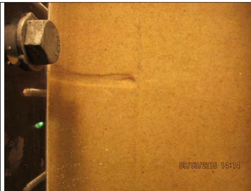
Figure 68-3 dent/impression in sand surface that slowed tip down
