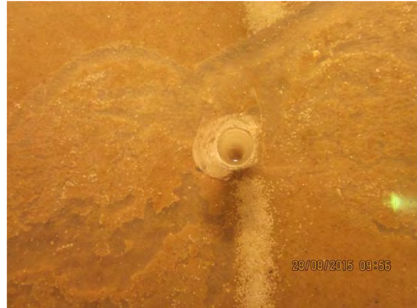
Figure 80-3 Wax filled hole and didn't flow into channel.
