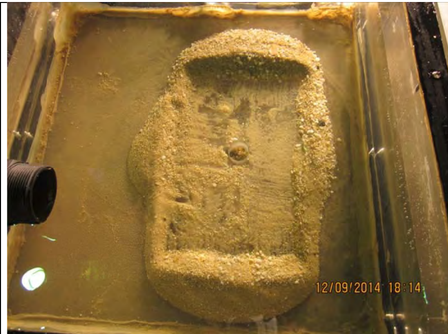
Figure 52-3 The same sand boil moved away from exit
