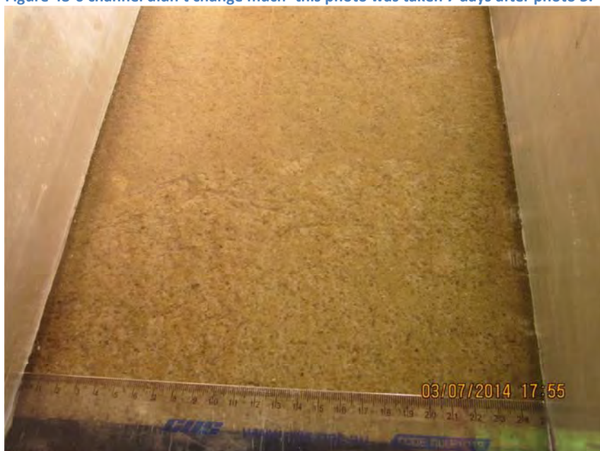
Figure 48-8 Coarse/"bony" appearance (possible evidence of suffusion)
