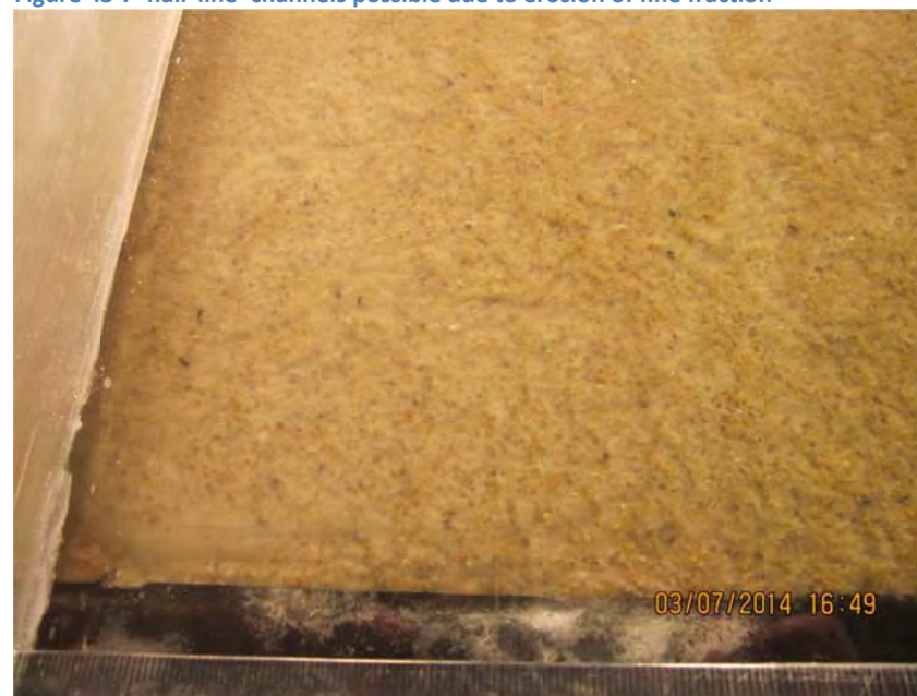
Figure 48-9 Cloudy water moving through sample (possible evidence of suffusion)
