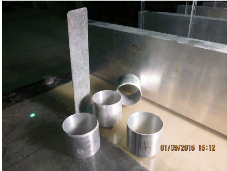
Figure 3.33: Density push tubes and ‘L’ shaped iron
