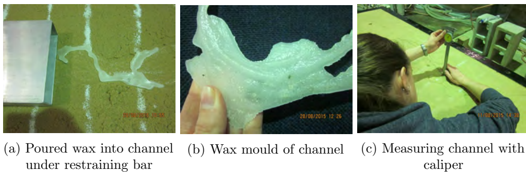
Figure 3.50: Measuring depth of channel
