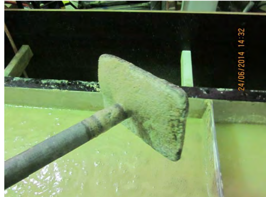
Figure 48-3 tamper became partially buried and when removed it lifted up soil with it
