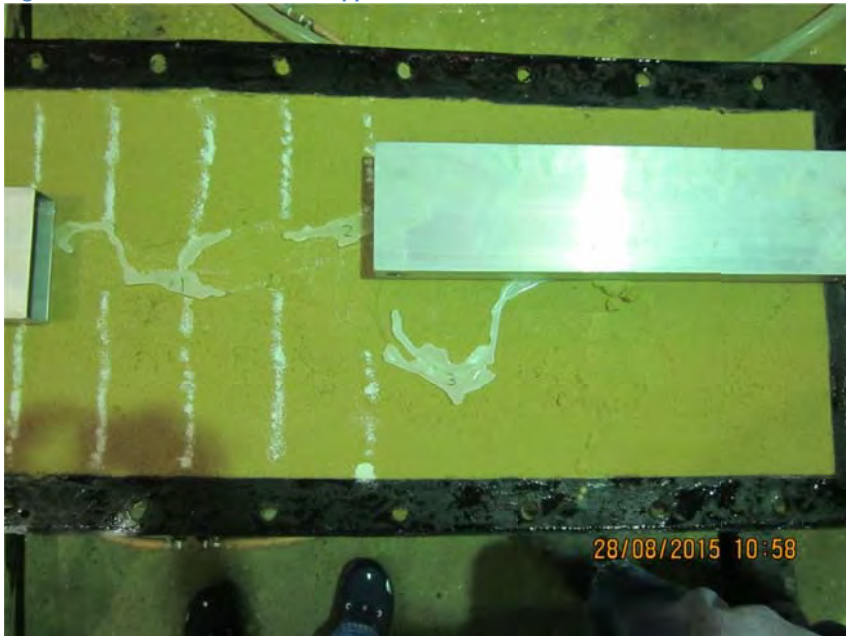
Figure 80-4 Wax poured beneath lid restraints and without cover
