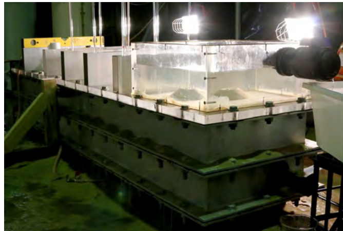
(c) Photo of oblique close-up (Note: there was only one sand boil, two can be seen due to refraction)
