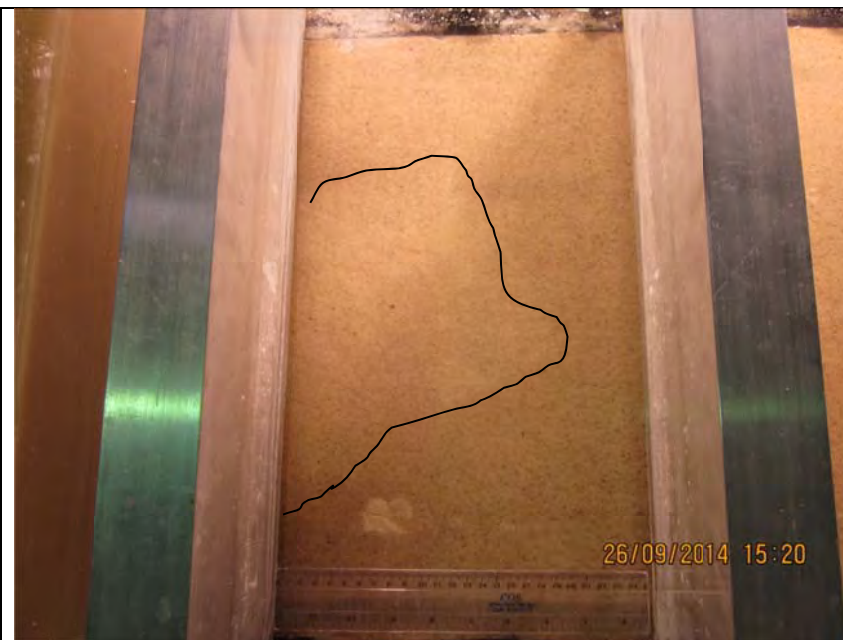
Figure 54-2 The start of failure by sheet flow (region indicated was slowly sliding d/s)
