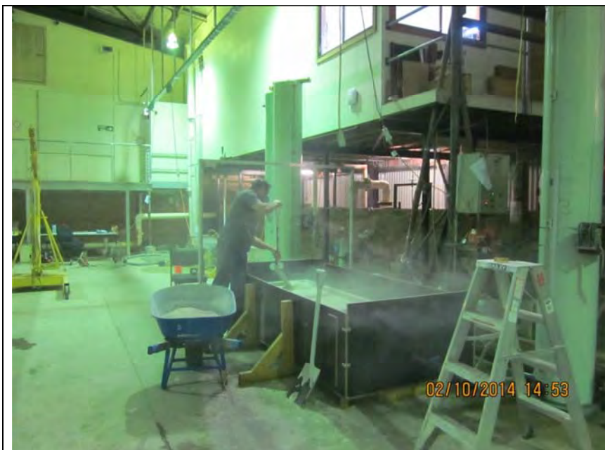
Figure 56-1 300g soil became airborne when tamping
