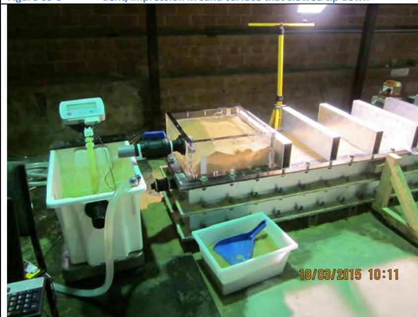
Figure 68-5 At end of exp showing the container full of sand removed from the exit (sand in the d/s box at time of pic was due to failure overnight)
