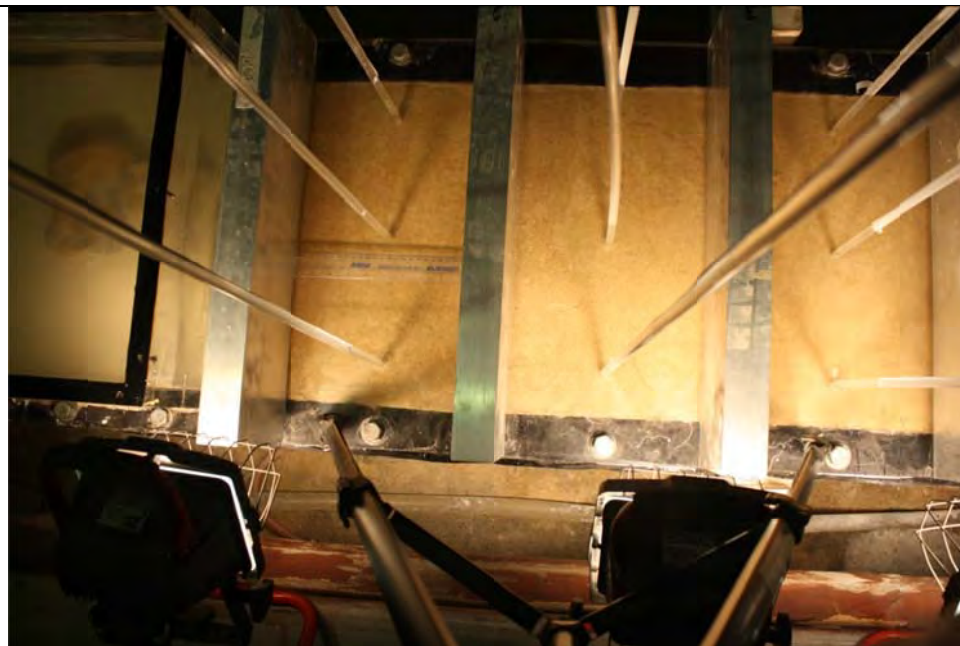
Figure 71-8 2 minutes before failure (discontinuous channel with "tip" at 640mm)
