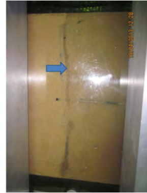
(b) Slope retreated and starter dowel pushed downstream (top of slope started in lower half of photo and dowel started further up)
