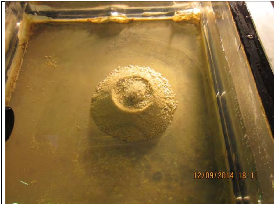
Figure 52-2 Sand boil when tip was 80ab1
