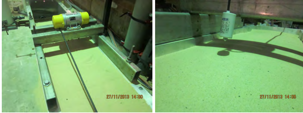
(a) Vibrator on steel frame
