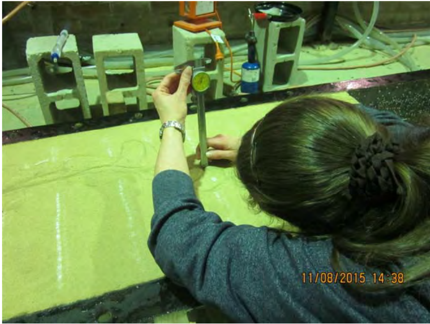
Figure 79-6 Measuring bare channel with calliper and fry pan in background
