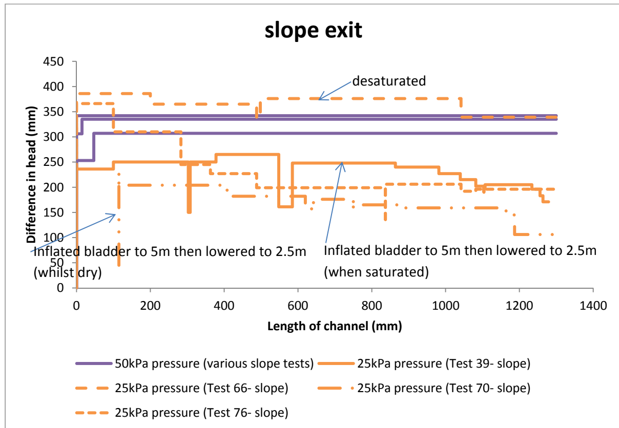
Figure 76-1 CL with head for test 76 and other slope tests
