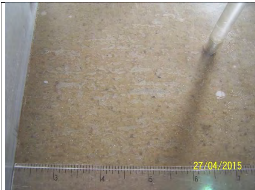
Figure 71-3 Bubbles in sample initially
