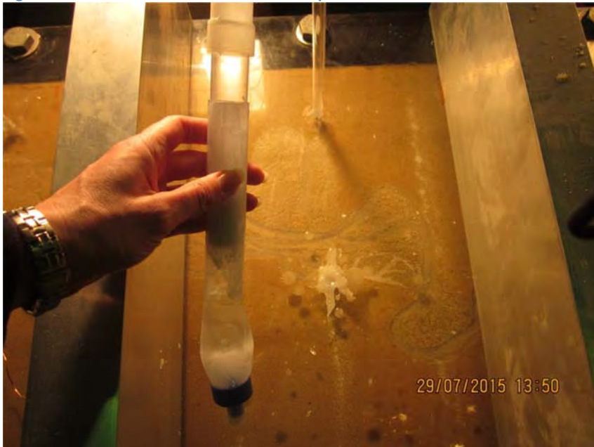
Figure 79-4 Plunger pushed wax into channel for about 50mm
