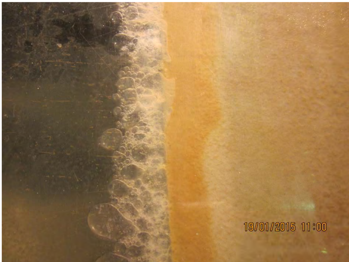
Figure 64-1 Soil discolouration along the upstream end
