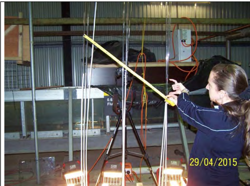
Figure 71-7 tape measure shows gradient btw rows 3 and 2 and my hand indicates level in row 1.
