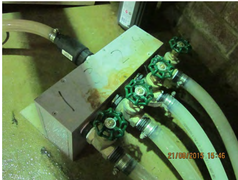
Figure 3.16: Manifold box used to split treated water from pit to four constant head tanks
