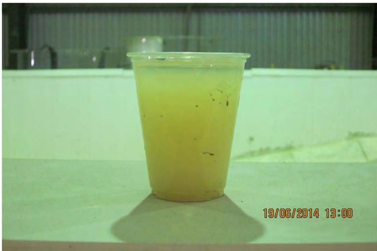
Pic 5: same water 4 hours later (fines don't settle)
