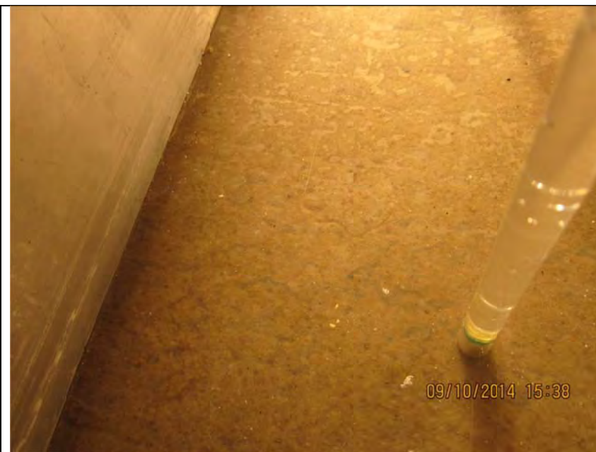
Figure 56-2 The pump had stopped during saturation so the water level dropped below the lid and air was brought into the sample
