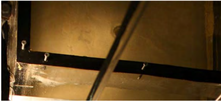
Figure 82-2 first sand boil before it was collected showing exit shaft was not full of sand
