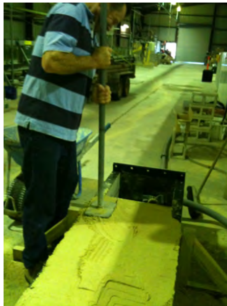
Figure 3.23: Tamper used to compact sample
