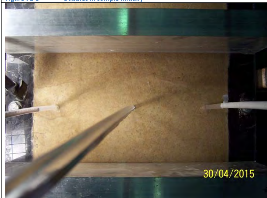
Figure 71-5 day 4-'tension crack' line had moved d/s
