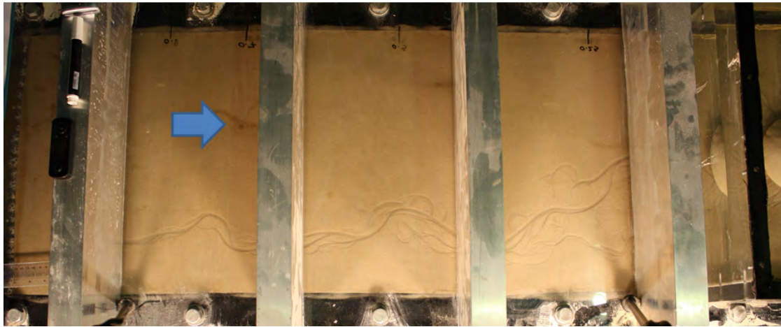
(c) Example of more channel meandering in uniform soil and more meandering and braiding toward downstream end (Test 57 in Sibelco 50n)
