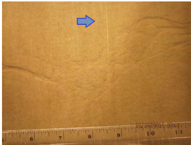
(b) Close up of blockage between enlarged and regular channels (Test 57 in Sibelco 50n)
