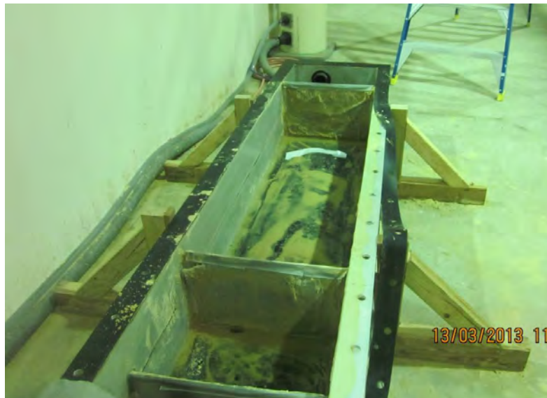
Figure 3.4: Empty flume showing inflated pressure bladder and internal panels lined with geofabric
