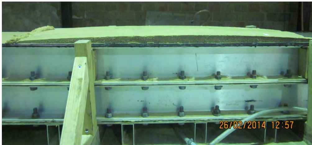
(c) Sand pushed up out of flume by bladder after Test 40
