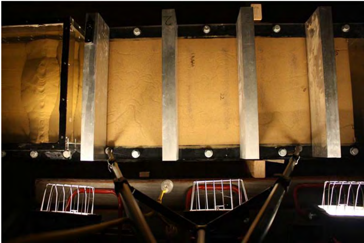
This photo shows the sand discolouration at the u/s end.
