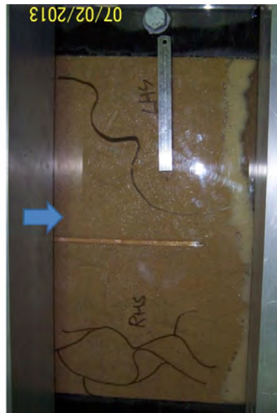
Figure 3.14: Plan view of organic build-up along downstream slope (along right-hand-side of photo) (blue arrow indicates direction of flow)
