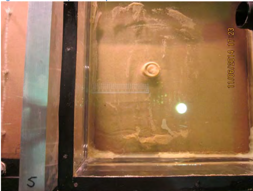
Figure 46-3 sand downstream of hole not pushed up against lid and channel 'A' initiated LHS (not from hole)
