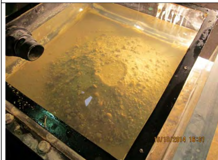
Figure 58-15 'channel' was wide so a lot of material transported down channel
