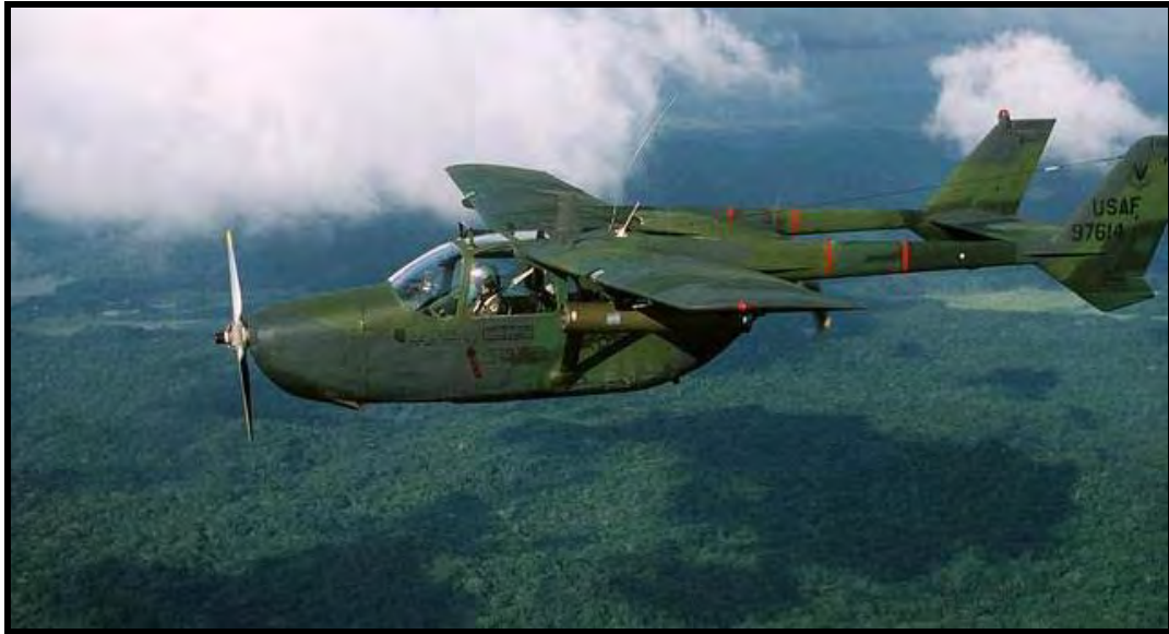
Photograph 32 : United States Air Force O2A Push /Pull Cessna 'Skymaster' aircraft. The O2B model is the same aircraft but without the forward air controller rocket pods under the wing. On the left-hand side behind the pilot built into the fuselage was an external speaker for broadcasting.
