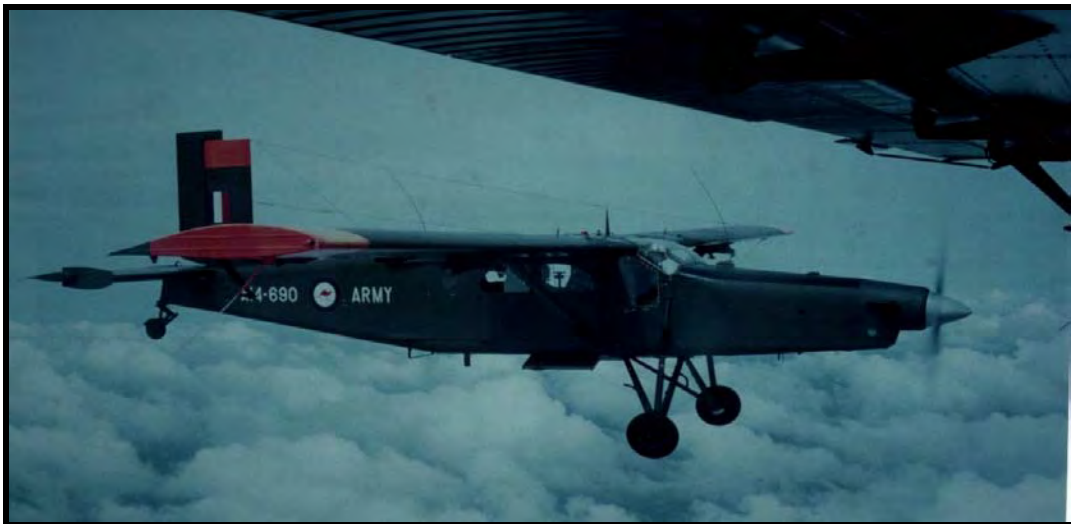
Photograph 33 : Pilatus Porter aircraft with underneath hatch open. This is where the broadcast speakers protruded from the aircraft.
