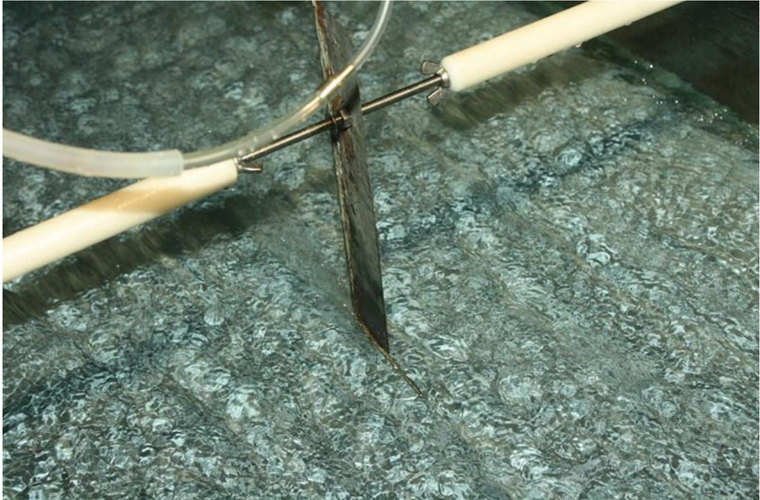
**FIGURE 3-13.** PITOT TUBE MEASUREMENTS IN FULLY DEVELOPED FLOWS DOWNSTREAM OF THE SLUICE GATE; NOTE THE FREE-SURFACE ROUGHNESS IN THE HIGH-VELOCITY FLOWS ( $Q = 0.059 \text{ m}^3/\text{s}$ ,  $h_0 = 0.03 \text{ m}$ ).
