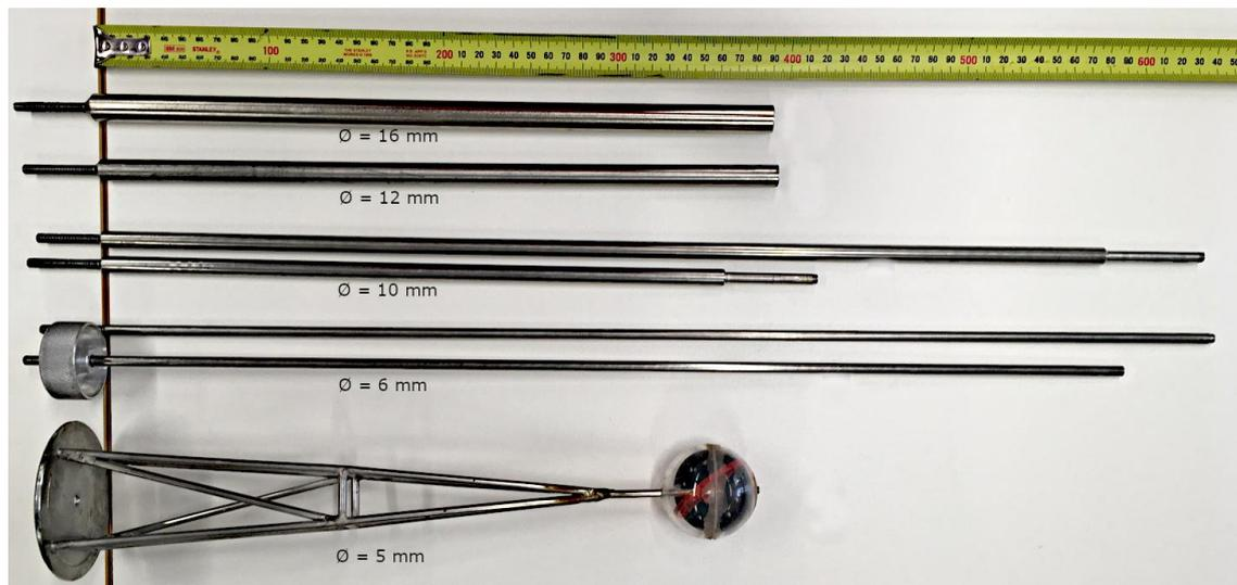
FIGURE H-1. DIFFERENT ROD DIAMETERS AND LENGTHS TESTED IN THE PRESENT STUDY.
