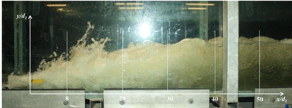
A) EXPERIMENT E:  $Fr_1 = 8.5$ ,  $Re = 7.5 \times 10^4$ ,  $x_{sg} = 1.66$  m,  $\delta = 0.03$  m - FULLY DEVELOPED INFLOW CONDITIONS
