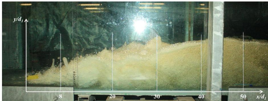
B) EXPERIMENT E:  $Fr_1 = 8.5$ ,  $Re = 7.5 \times 10^4$ ,  $x_{sg} = 0.5$  m,  $\delta = 0.01$  m - PARTIALLY DEVELOPED INFLOW CONDITIONS
