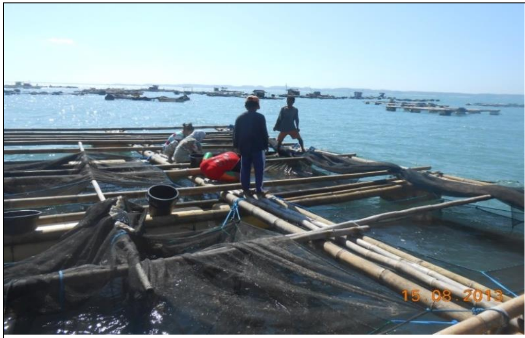
Figure 2.9. The commonly used unit of floating sea cages, with several cages of 3 \times 3 \times 3 m. A unit of floating sea frames usually consists of 9 cages (243 m 3 total volume).
