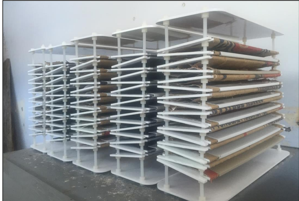
Figure 6.5. Experimental crevice collector made to test different substrate materials and crevice angles in the tank experiments
