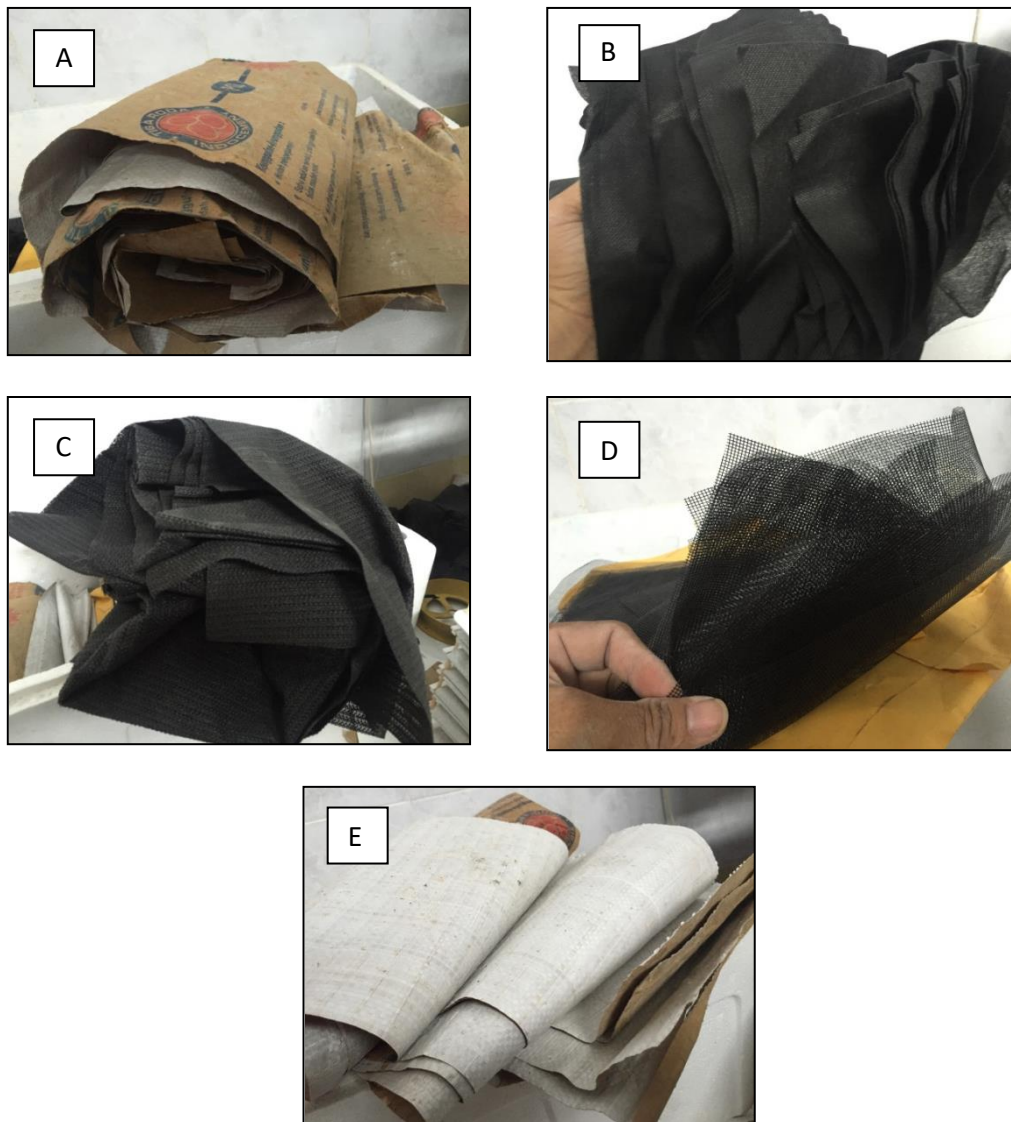
Figure 6.1. Materials used for the collectors in the tank experiment: A, cement bag paper; B, weed fabric; C, PVC rubber; D, insect mesh; E, cement bag plastic
