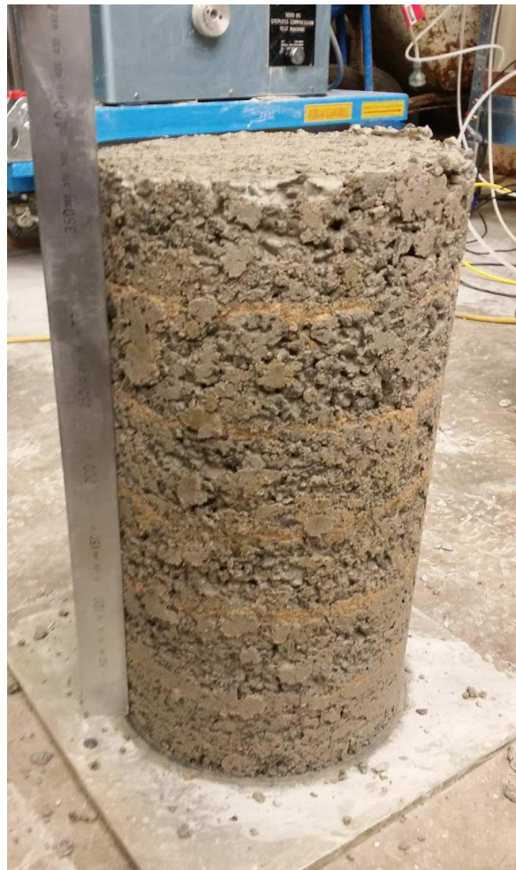
Figure 3-15 A photo of compacted soil sample with dry sand mark.
