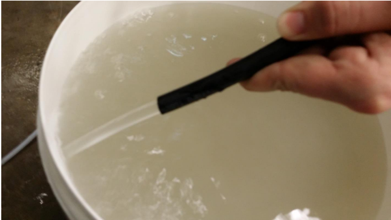
Figure 4-10 Photo of effluent at the early stage of internal erosion.
