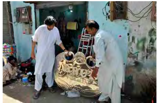
Figure 2.64b: Syed M I, Abdullah. 2012. First prototype for Brut for Men sculptures. Prototype failed. Incorrect dimensions and wrong steel gauge rendered an un-satisfactory result. Photo: Fahim Rao.
