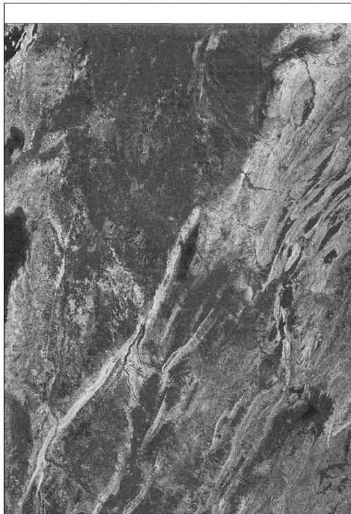
Figure 2.6 The coherence map corresponding to the interferogram in Figure 2.5
