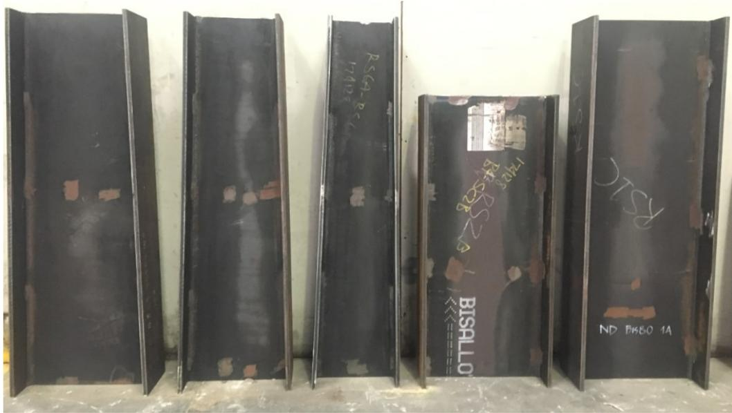
**Figure 3.7:** Prismatic and tapered residual stress specimens.
