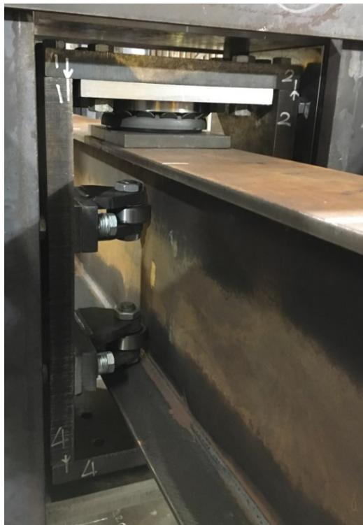
**Figure 4.11:** Loading box: (1) outer box, (2) inner box, (3-5) roller bearings, (6) spherical roller bearings, (7) modified spherical thrust roller bearing, and (8) I-beam specimen.
