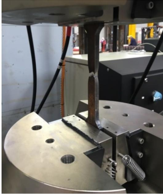
**Figure 3.11:** Tensile coupon test.
