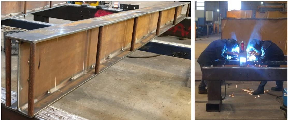
**Figure 3.6:** Fabrication procedure of residual stress specimens.
