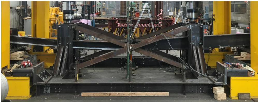
Figure 5.4: LTB test set-up for web-tapered beams.
