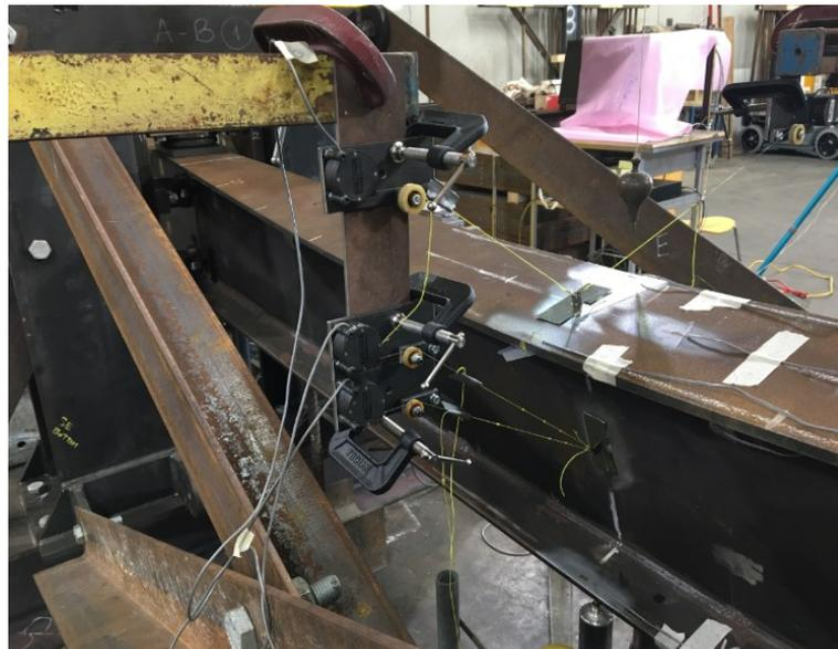
(b) Draw-wire transducers tracking the movement of the beam centroid and top-flange centre.
