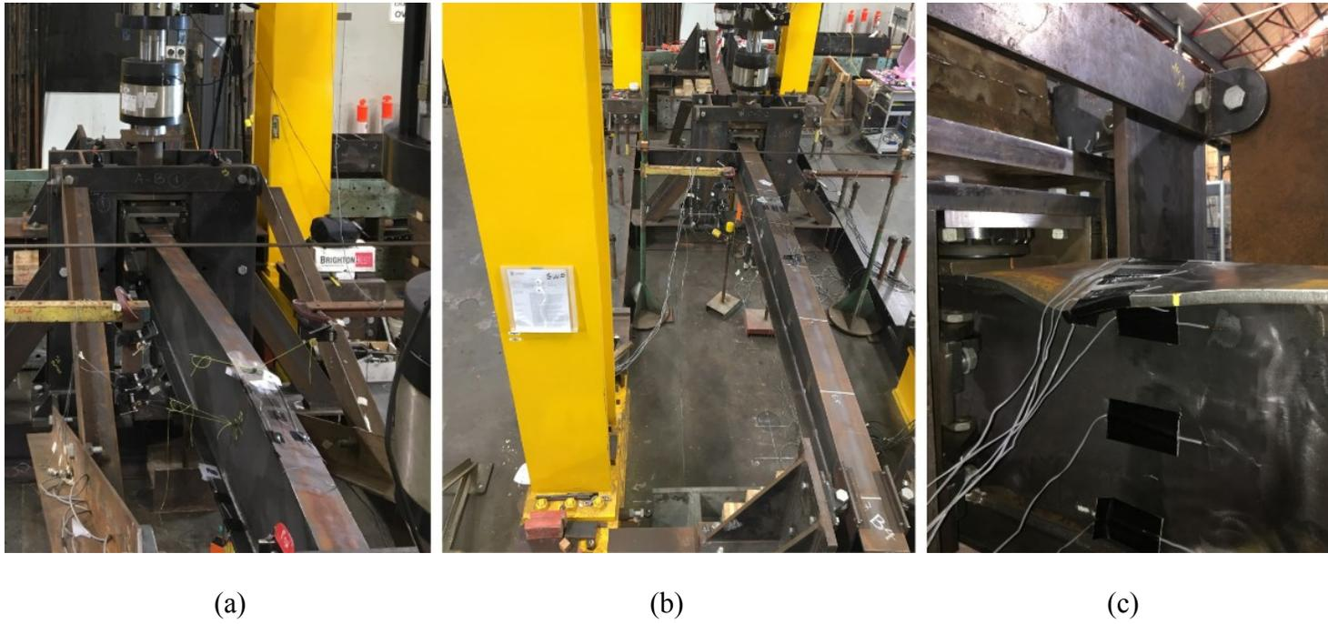
**Figure 4.19:** Buckling modes: (a) LTB of an I-beam under UM, (b) LTB of an I-beam under MG, and (c) FLB of an I-beam under UM.
