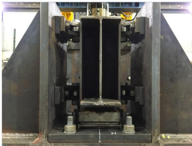
**Figure 5.6:** End restraint in the test of web-tapered beams
