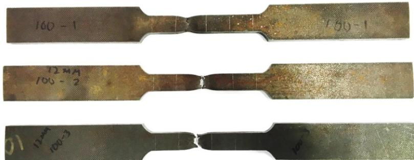
**Figure 3.12:** Tensile coupons of 12 mm BISPLATE-100 plates.
