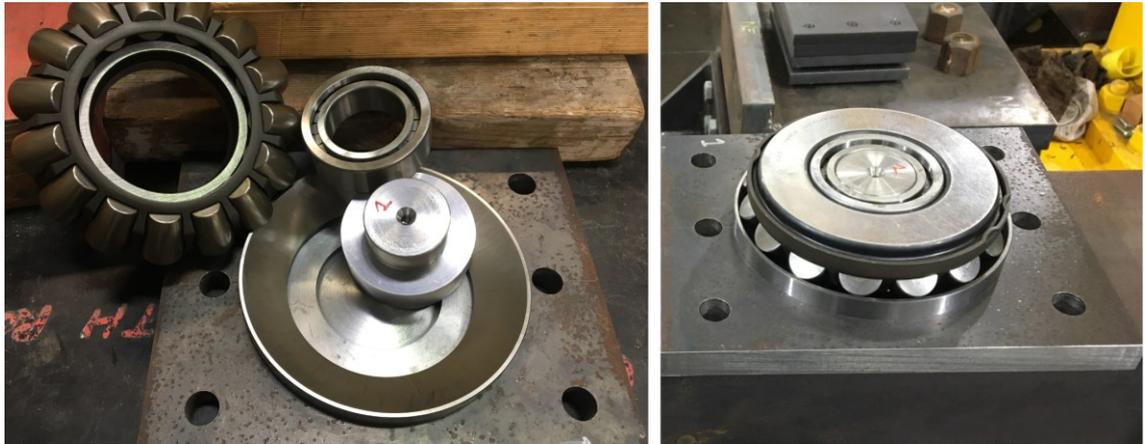
(a) The modified spherical thrust roller bearing
