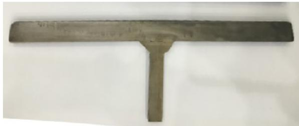
**Figure 3.8:** BISPLATE-100 stress-free reference sample.
