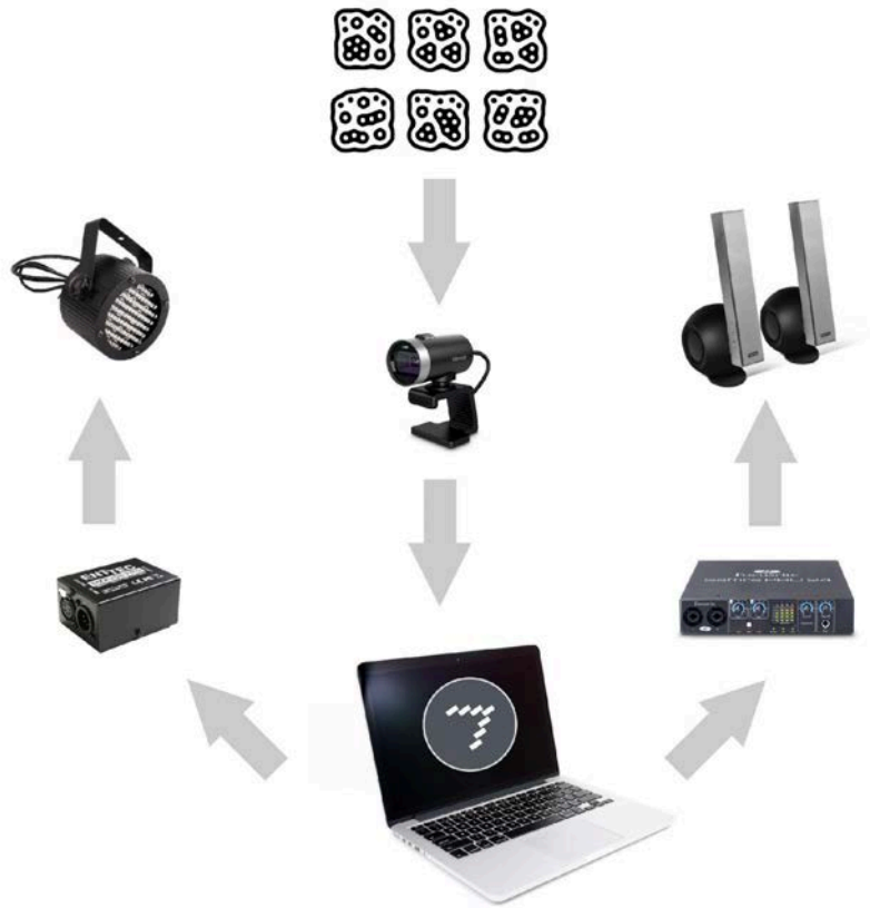
Figure 3.17 - Flow of input/output in the Responsive Dome Environment (Iteration 1).
