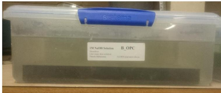
Figure 3-27 : Mortar bars kept in 1M NaOH solution
