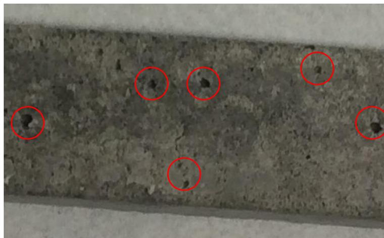
Figure 5-12 : surface holes identified in mix 2
