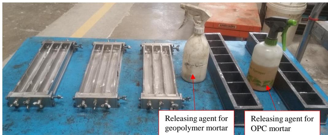
Figure 3-21 : Moulds ready for casting
