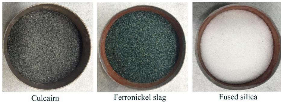
Figure 4-1 : Aggregates (0.6mm-0.3mm) prepared for testing
