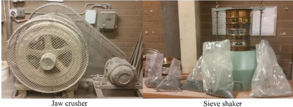
Figure 3-19 : Jaw crusher and sieve shaker used to prepare aggregate
