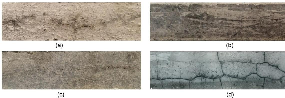
Figure 6-16 : Mortar bar images of mix 1-4 after the test (150 days); (a) Mix 1 at 150 days, (b) Mix 2 at 150 days, (c) Mix 3 at 150 days, (d) Mix 4 at 150 days
