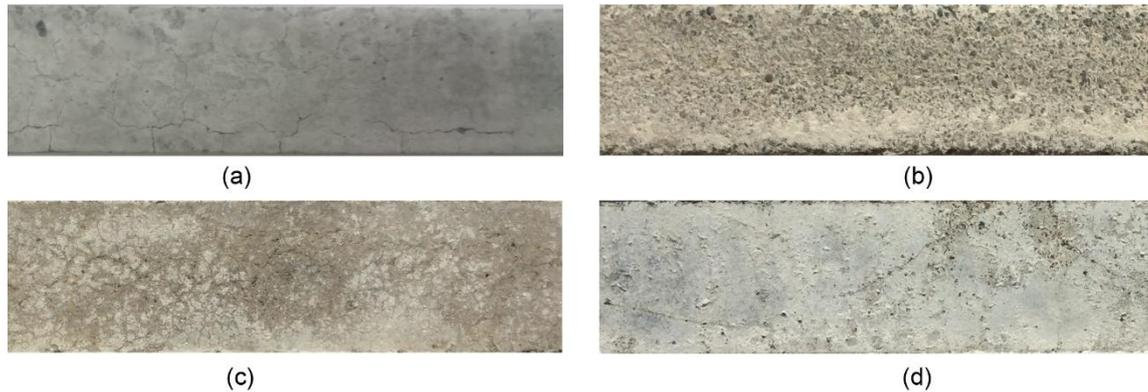
Figure 7-17 : Mortar bar images of mix 1-4 after the test (150 days); (a) Mix 1 at 150 days, (b) Mix 2 at 150 days, (c) Mix 3 at 150 days, (d) Mix 4 at 150 days
