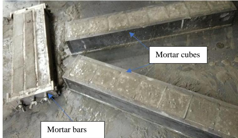
Figure 3-25 : Compacting the specimens with a vibration table
