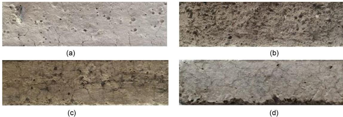
Figure 8-17 : Mortar bar images of mix 1-4 after the test completion; (a) Mix 1 at 21 days, (b) Mix 2 at 150 days, (c) Mix 3 at 150 days, (d) Mix 4 at 150 days
