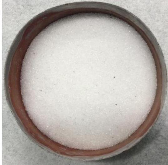
Figure 3-15 : Fused silica slag aggregate prepared for a mix
