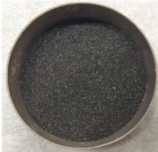
Figure 3-6 : Basalt aggregate prepared for a mix
