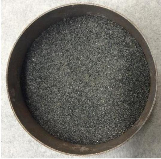
Figure 3-9 : Culcairn aggregate prepared for a mix
