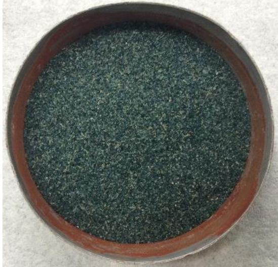
Figure 3-12 : Ferronickel slag aggregate prepared for a mix
